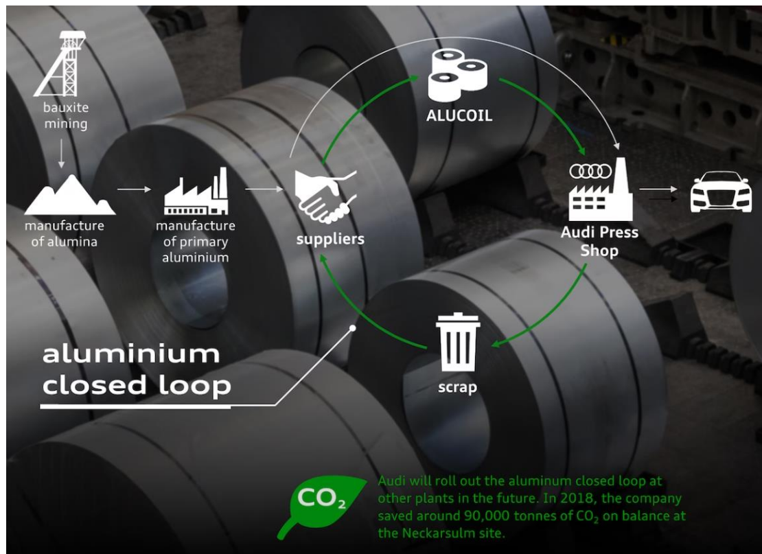
4-2. Figure_ Audi's Aluminium Closed Loop
