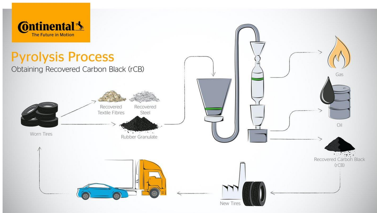
4-6. Figure_Pyrolysis process at Continental: recovered carbon black (rCB).
