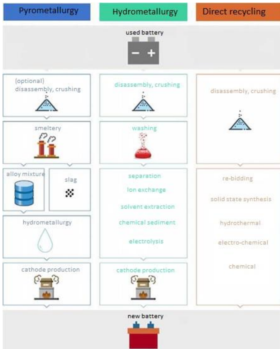
Figure 22 - Recycling processes of lithium-ion batteries
