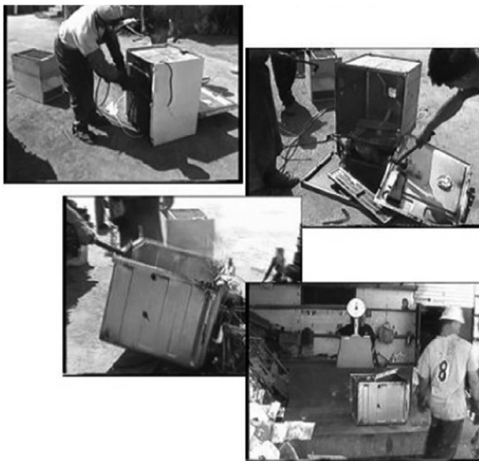
10. Figure_ Manual disassembly of the dishwasher [Source: Kandikjan, 2006]
