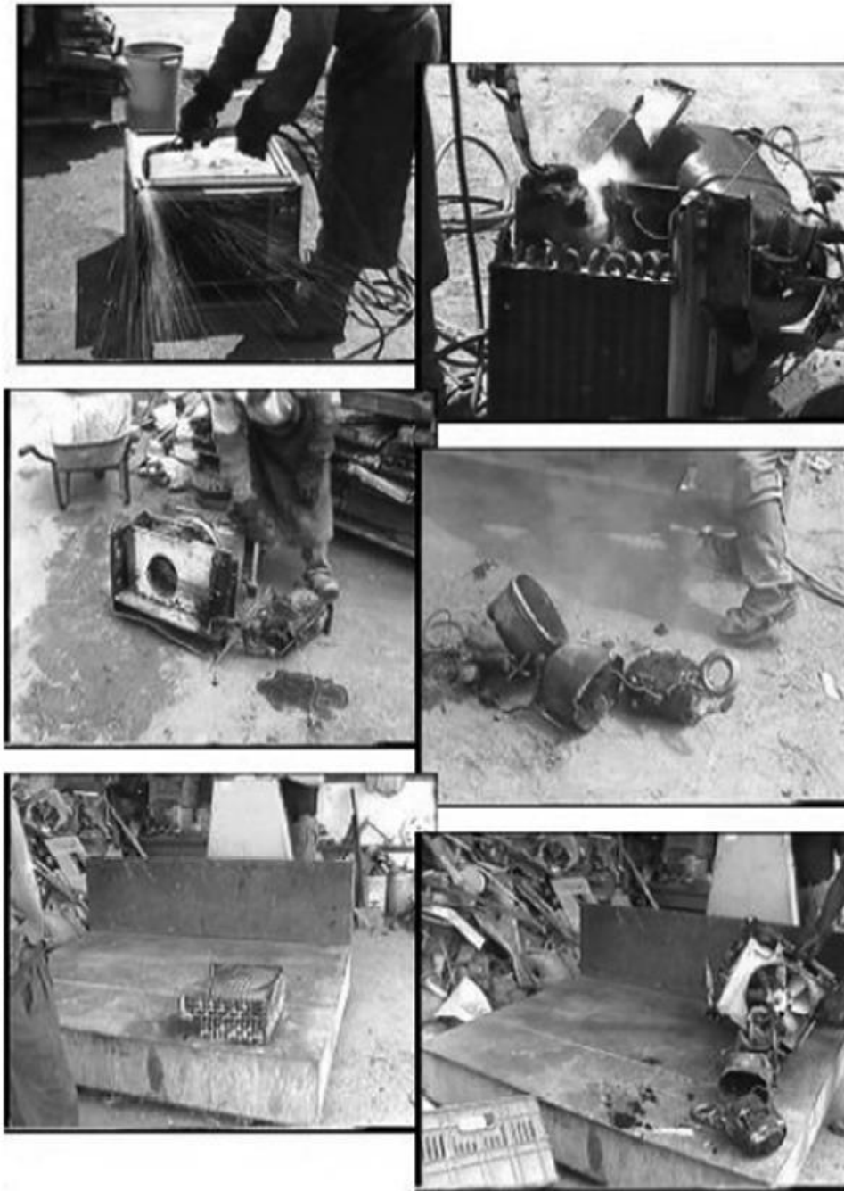
11. Figure_ Manual disassembly of the air-conditioner [Source: Kandikjan, 2006]
