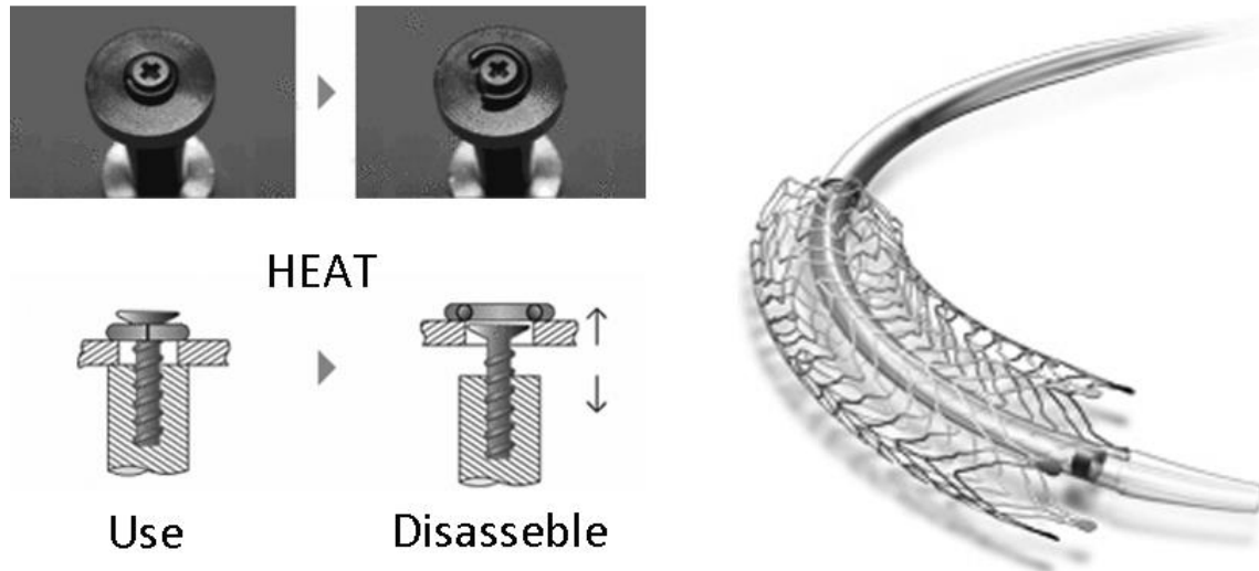
5. Figure_Disassembly by heating the component with screw connection and Nitinol washer (left) and Nitinol stent after heating (right)
