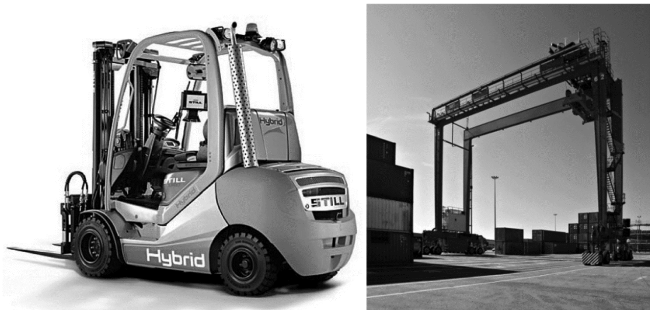
14. Figure_Transport machinery: Hybrid powered forklift (left) and ECO E-RTG electrically powered crane (right)
