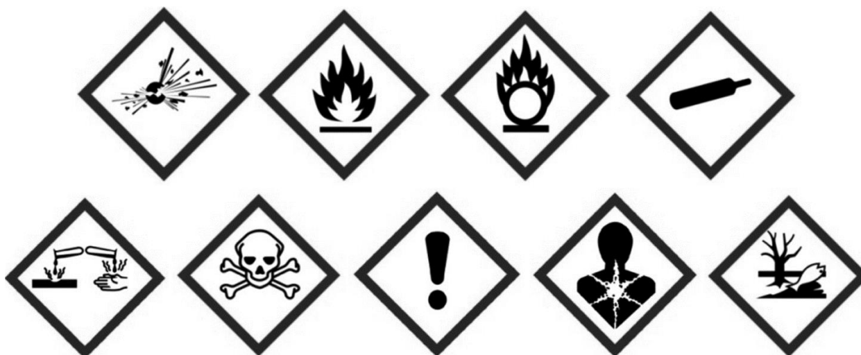
68. Figure_Symbols for explosive, flammable and oxidizing substances, pressurised gases, corrosive, toxic and substances harmful for the respiratory system and nature (respectively)
