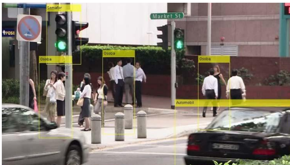
1-23. Figure Software for the recognition of traffic participants as a result of the Master's thesis in the Department of Motor Vehicles
