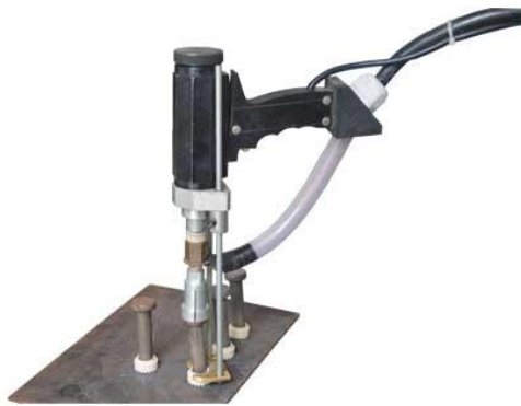
Figure 28. Welding gun and welded studs with ceramic rings [24]
