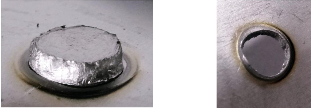
Figure 20. Pulled out resistance spot welded seam
