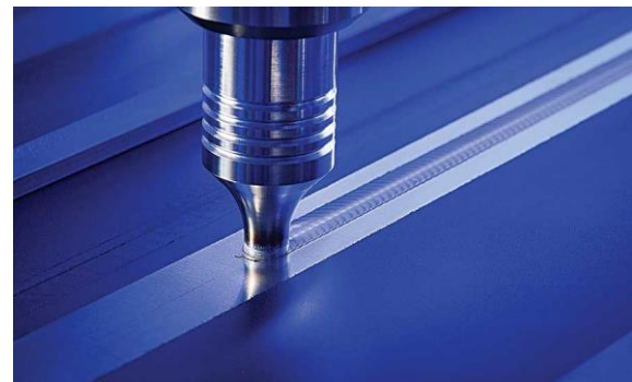
Figure 12. Tool during welding [9]
