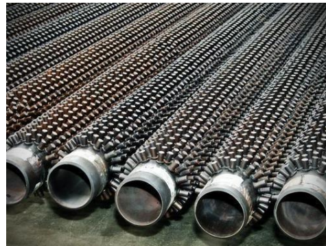
Figure 29. Welded studs on boiler tubes [25]
