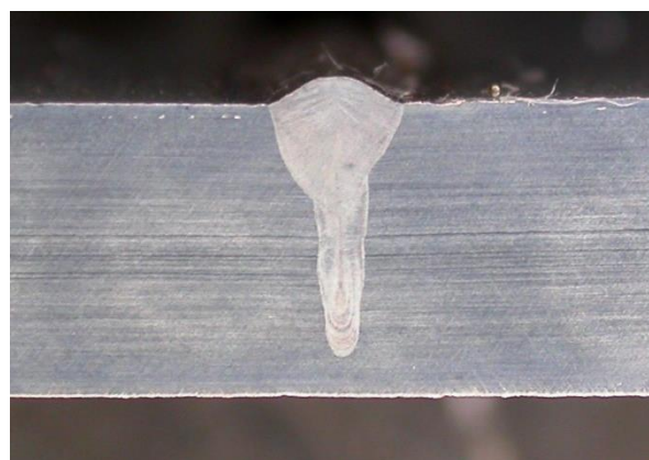
Figure 64. Deep penetration weld using a 5 kW CO 2 laser, s=5 \text{ mm}
