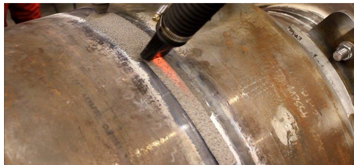
Figure 37. Welding of a rotating vessel with submerged arc [31]
