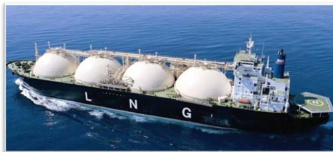
The LNG carrier Aristidis I. transporting liquefied natural gas in spherical containers.
