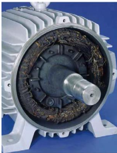
4-69. Figure Burned wire insulation due to long term over-current [12]
