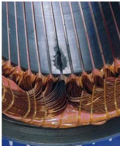
4-67. Figure Short circuits between winding and stator core inside the stator slot
