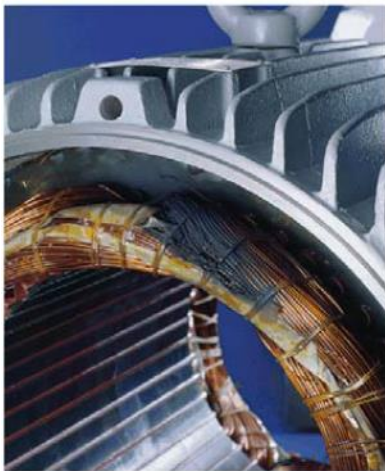
4-63. Figure Short circuit between phases [12]
