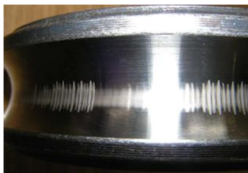
4-73. Figure Damaged bearing rolling surface
