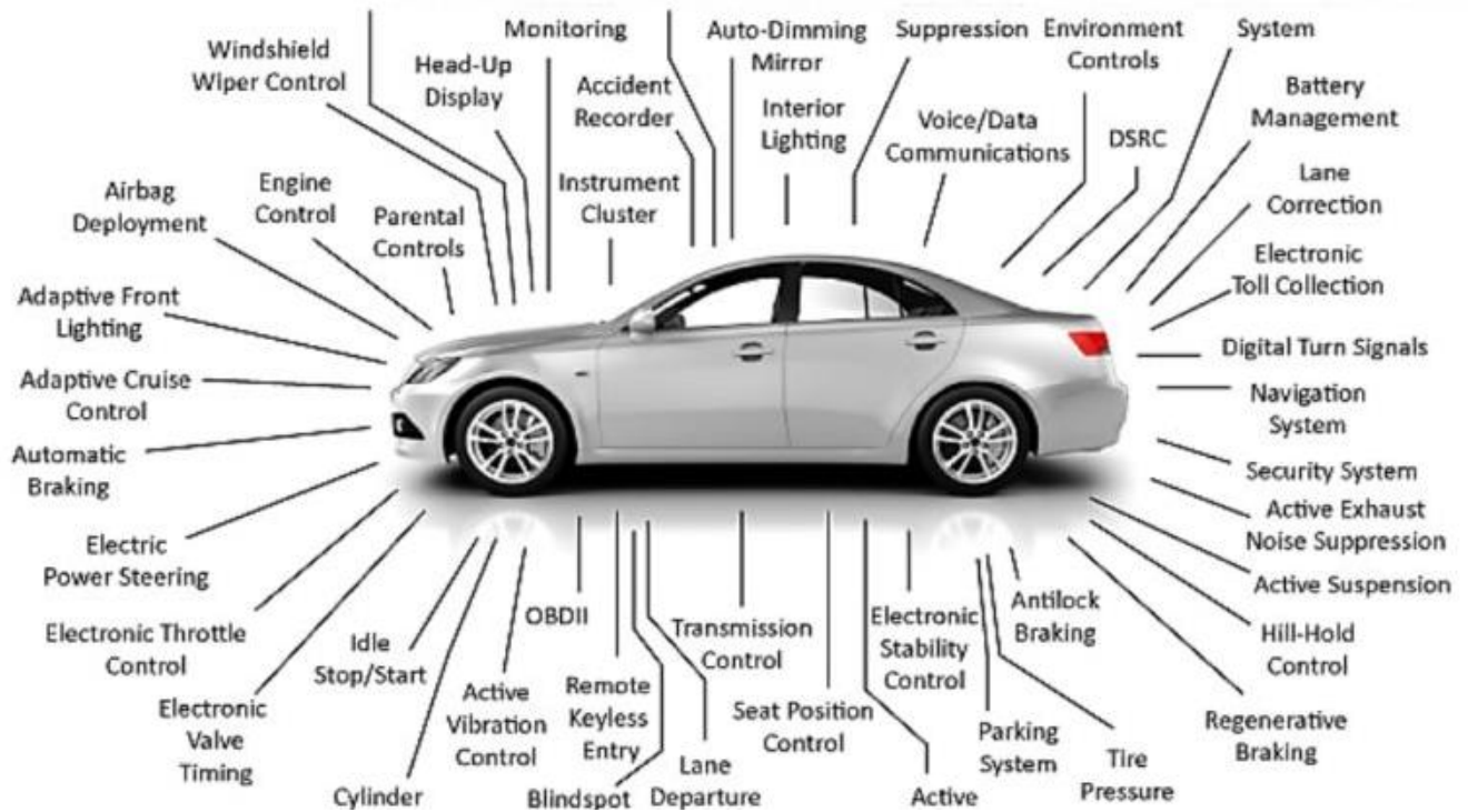
4-18. Figure_Role of Electronic Control Units in vehicle performance
