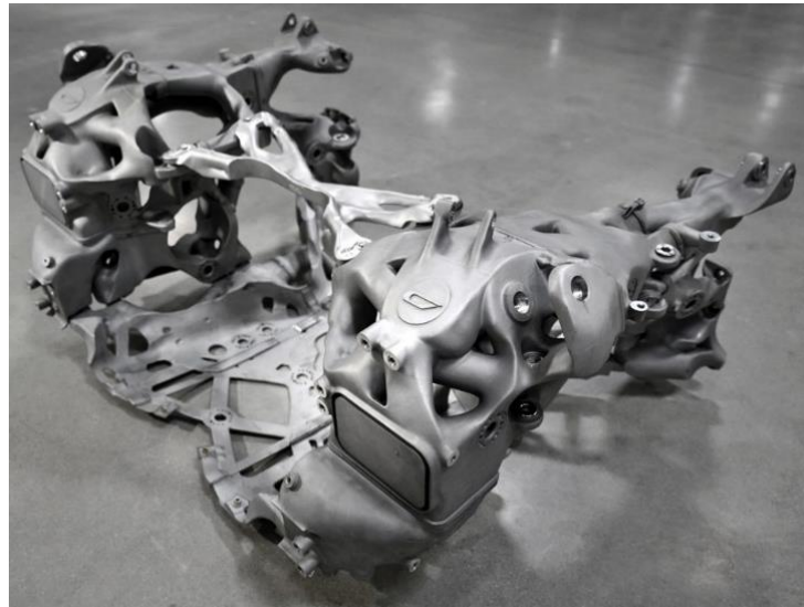
11-4. Figure_ The assembled rear structure, showing the extent to which metal Additive Manufacturing has been used on the 21C [Source: Czinger Vehicles]
