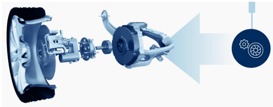
4-12. Figure_ The in-wheel motor system
