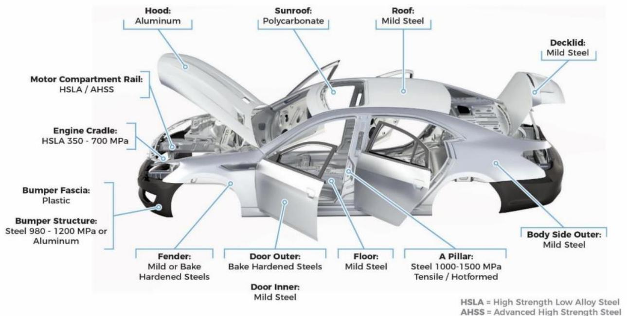
1-5. Figure\_ Materials Used Most Commonly for Major Vehicle Structure Components in the Current Fleet
