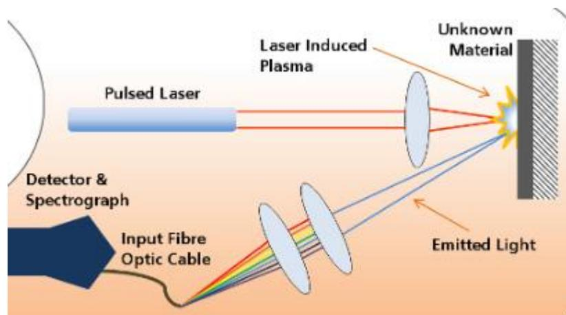
1-10. Figure\_ Laser-induced breakdown spectroscopy (LIBS)
