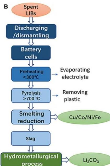
5-6. Figure\_((B) Pyrometallurgical process
