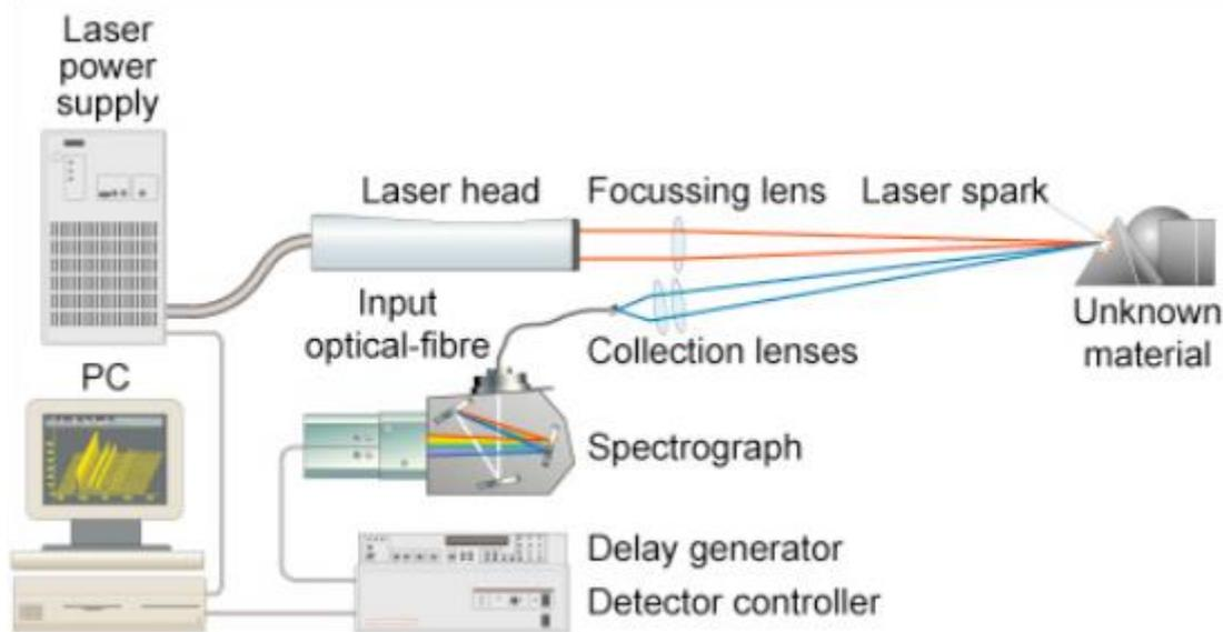
1-11. Figure\_ Schematic illustration of LIBS detection
