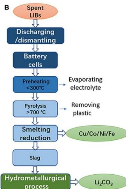
5-6. Figure\_(B) Pyrometallurgical process
