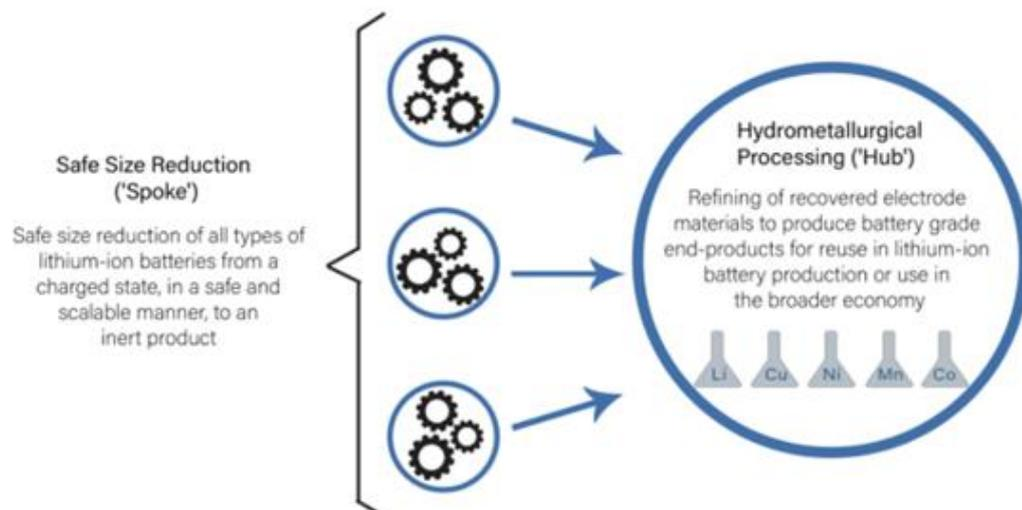
Figure 5-12: „Spoke and Hub” Method from Li-Cycle
