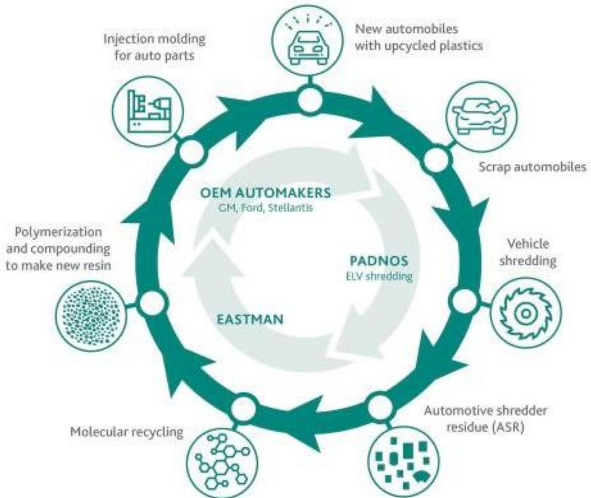
3-3. Figure\_Closed-loop recycling of automotive mixed plastic waste
