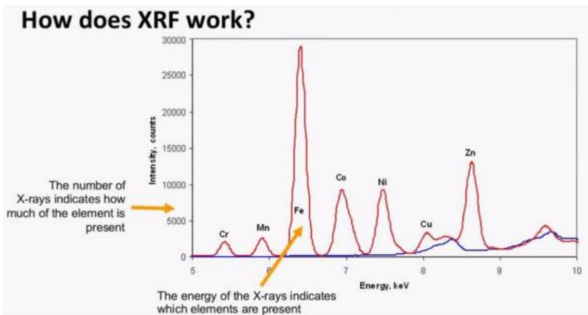
1-13. Figure\_ Schematic illustration of XRF detection
