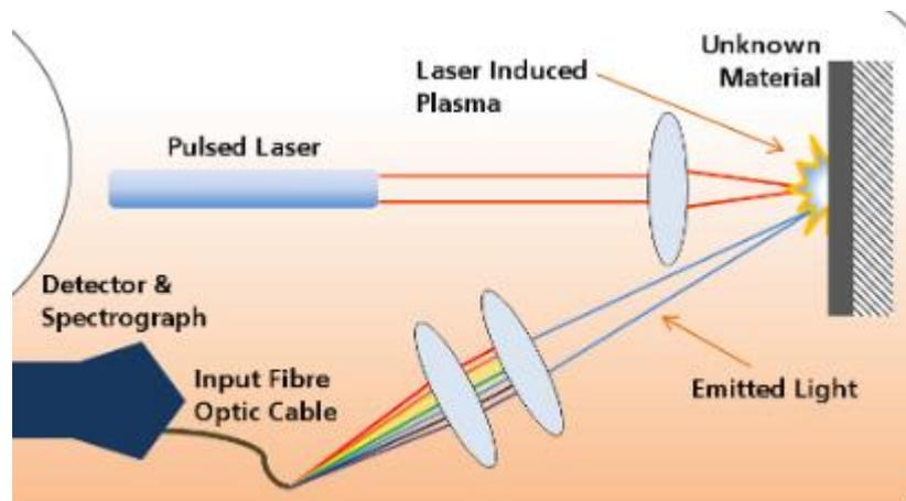
1-10. Figure\_ Laser-induced breakdown spectroscopy (LIBS)
