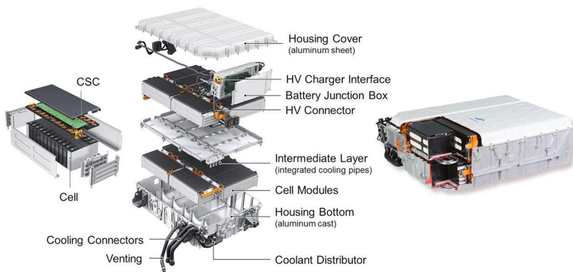
5-1. Figure\_Schematic build-up of an automotive battery system
