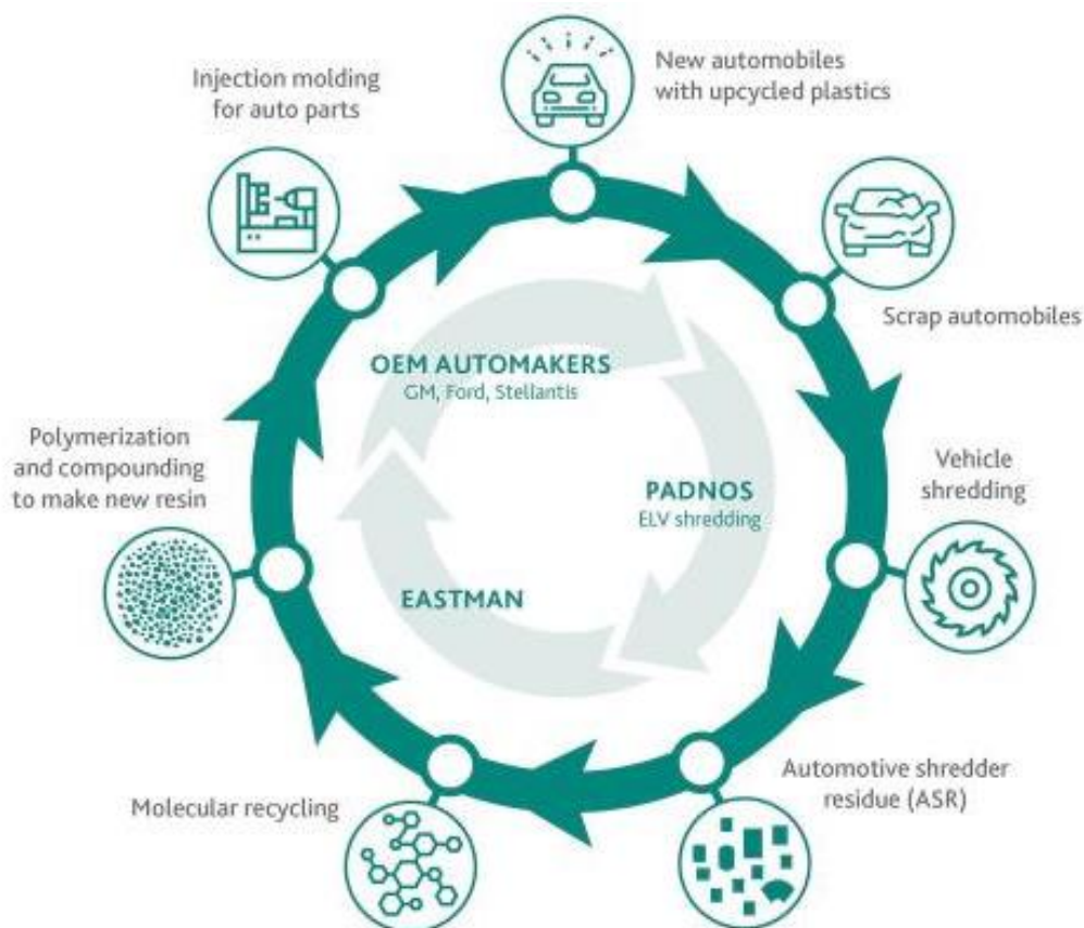
4-8. Figure_ Circular Economy from Eastman: Closed-Loop Recycling of Automotive Mixed Plastic Waste
