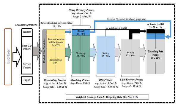
4-10. Figure\_ Process material flow diagram [21]
