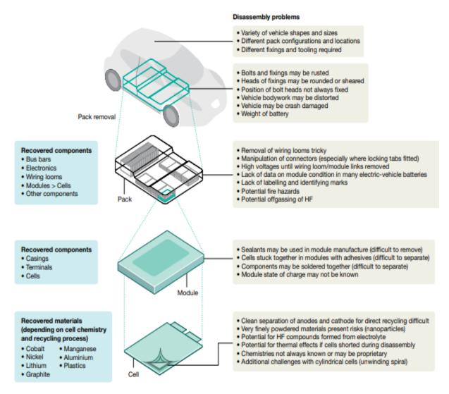
5-9. Figure\_ Diagram showing the takedown challenges at different levels of scale [32]
