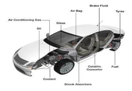
4-3. Figure\_ Identification of hazardous fluids and materials [17]
