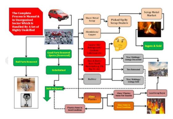
5-1. Figure\_ The recycling flow of a car [22]
