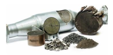
5-3. Figure\_ Catalytic converter recycling [25]
