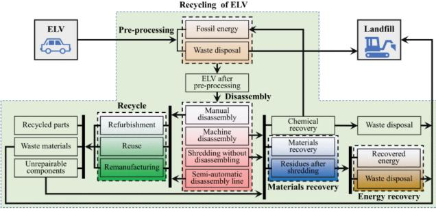
1-3. Figure\_Typical mode of ELV disassembly and recycling.
