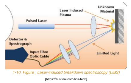
The laser is focused to form a plasma, which atomizes and excites samples. In principle, LIBS can analyze any matter regardless of its physical state, be it solid, liquid or gas.
