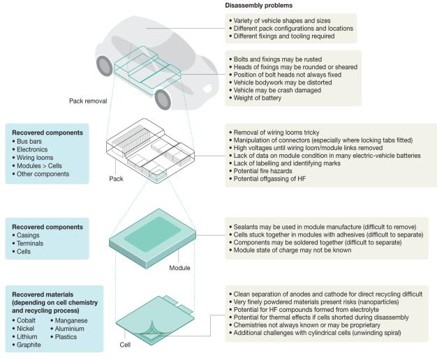
5-4. Figure\_Challenges of disassembly at different levels of scale
