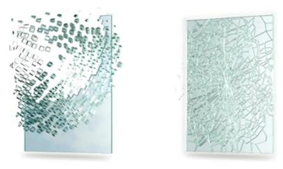
4-2. Figure\_ Tempered glass vs Laminated glass
