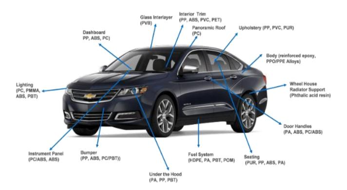
3-1. Figure\_ Plastics applications in automotive parts [http://adapt.mx/plastics-in-the-automotive-industry-which-materials-will-be-the-winners-and-losers/]
