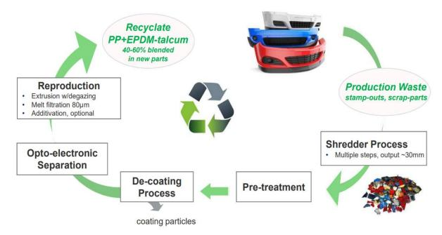
3-4. Figure\_ WIPAG – Closed loop recycling value chain >> bumper to bumper (PIR) [Source: https://circulareconomy.europa.eu/platform/sites/default/files/bsp\_albis\_wipag\_open\_loop\_closed\_loop\_raas\_10\_19s.pdf]
