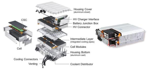
5-1. Figure\_Schematic build-up of an automotive battery system [Source: SAMSUNG SDI]
