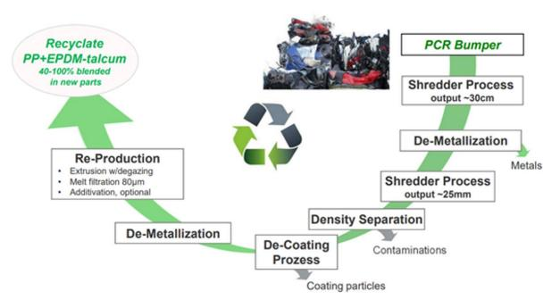
3-5. Figure\_ WIPAG – Closed loop recycling value chain >> bumper to bumper (PCR) [Source: https://circulareconomy.europa.eu/platform/sites/default/files/bsp\_albis\_wipag\_open\_loop\_closed\_loop\_raas\_10\_19s.pdf]
