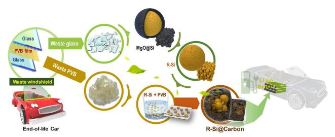
4-4. Figure\_Schematic of the synthesis method of reduced silicon and silicon/carbon composites for lithium-ion batteries
