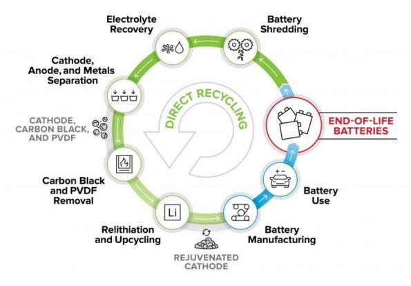
5-10. Figure\_ Direct Recycling - A schematic showing processes that a direct recycling process may include
