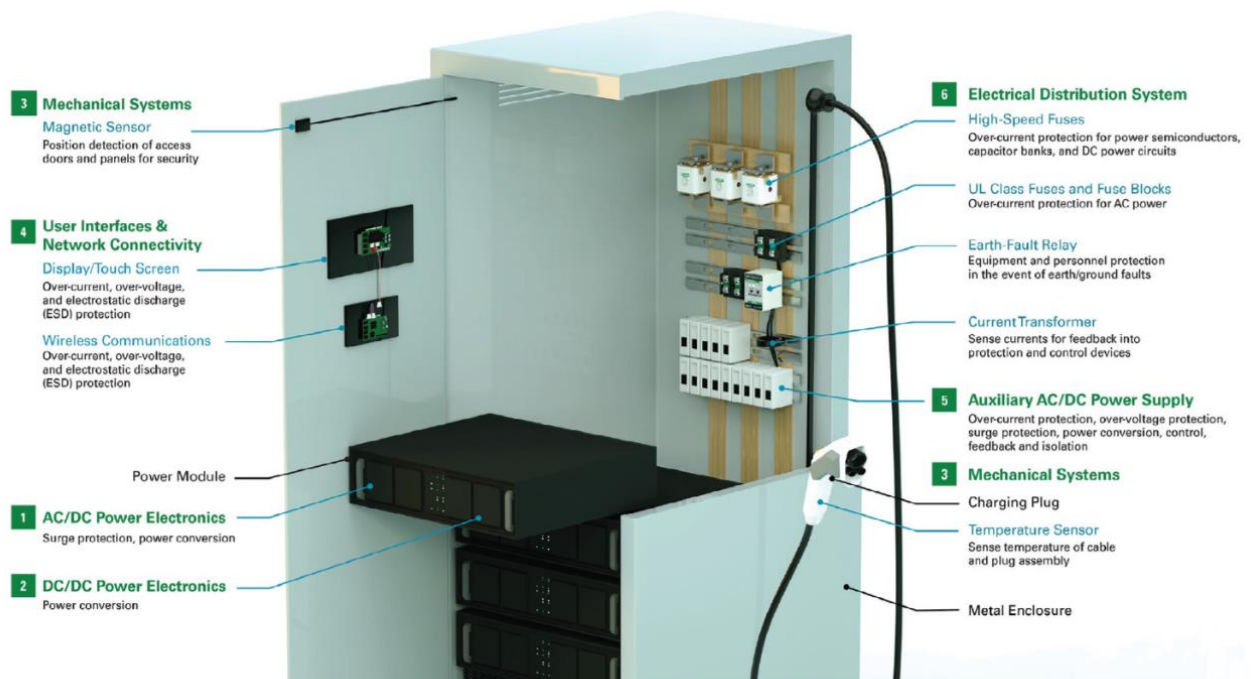
4-17. Figure_ Inside an EV charging station. (Source: TTI.)
