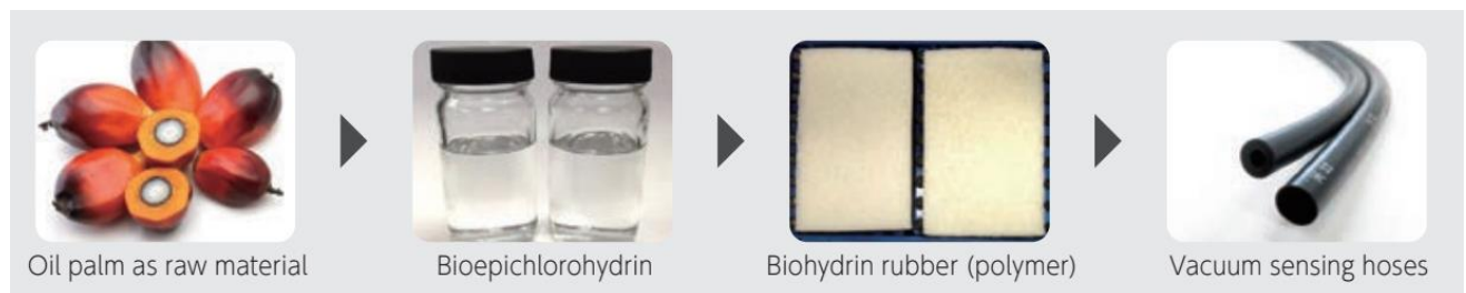
10-4. Figure_ Toyota became the world's first automaker to use biohydric rubber
